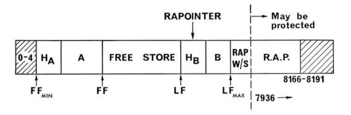
In the above diagram, assume that A and B are the first and second programs to be placed by RAP and that HA and HB are the locations which contain their respective 'Heads'. The five 'Head' locations contain the following details:
