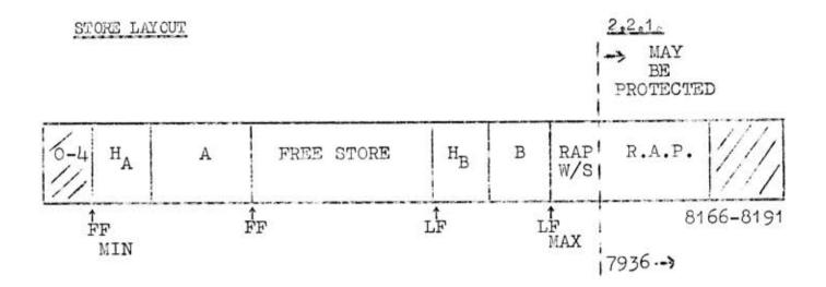
In the above diagram, assume that A and B are the first and second programs to be placed by the RAP and that HA and HB are the locations which contain their respective 'Heads'. The five 'Head' locations contain the following details:-
